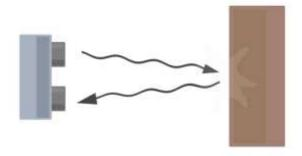
Diagram of the basic ultrasonic sensor operation **SERVO MOTOR:**
