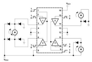
One H-bridge circuit is inside each L293D chip, and they can each turn a DC motor on their own. Due to its small size, it is widely used to power DC motors in robots. Here is a picture of how the pins on an L293D motor driver are set up.
